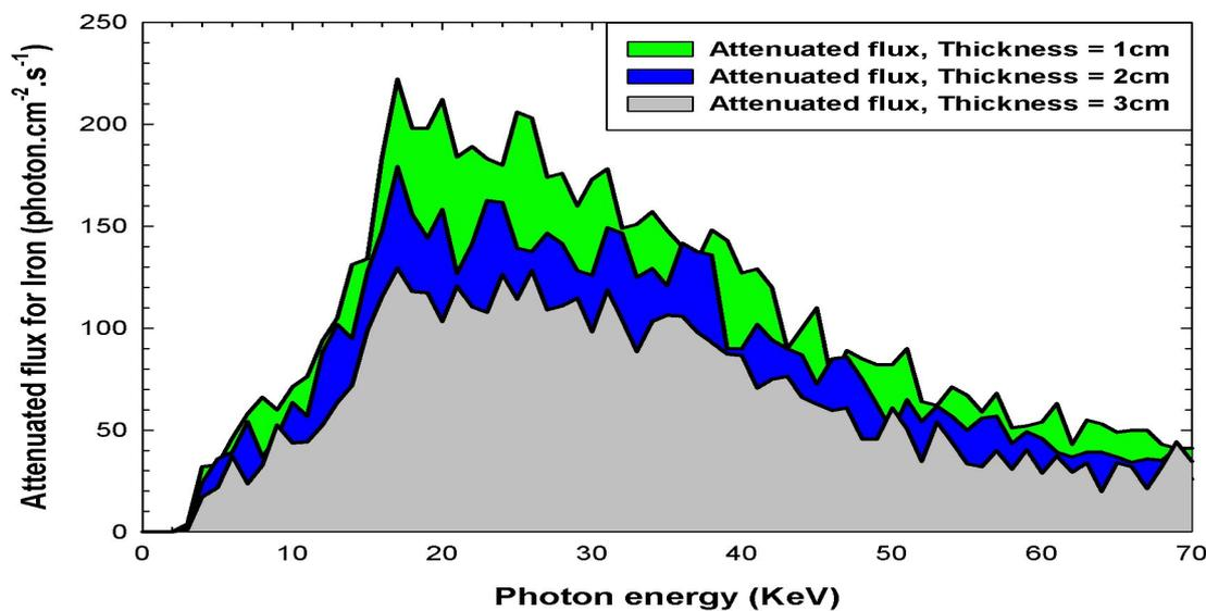
Fig.(1-d). Transmitted intensity as a function of thickness for Iron
